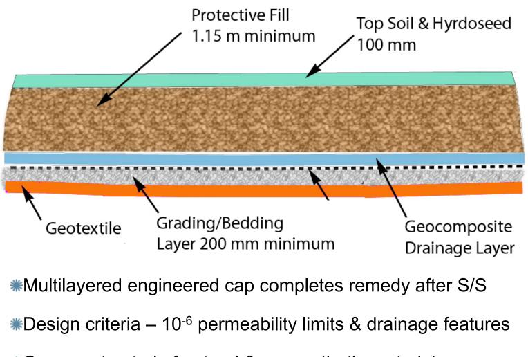
Cap constructed of natural & geosynthetic materials
