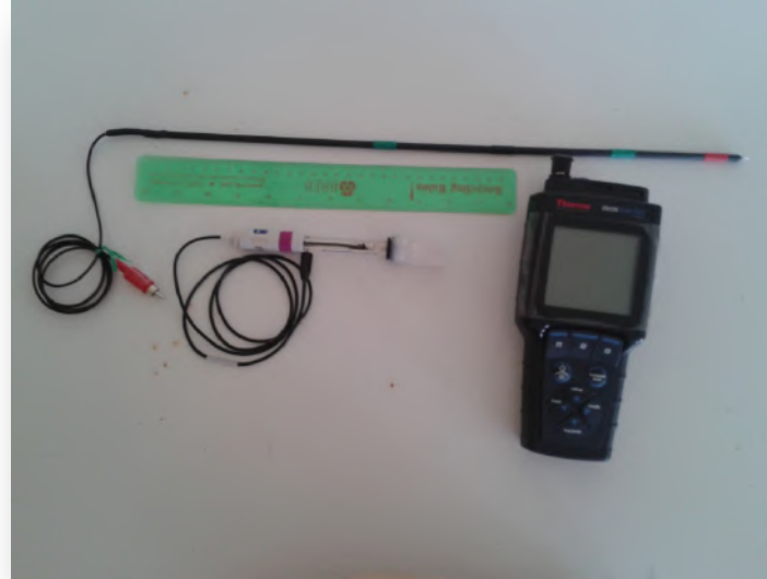
Millivolt meter, platinum tipped probe & Calomel reference electrode (C. Skinner, 2013)
